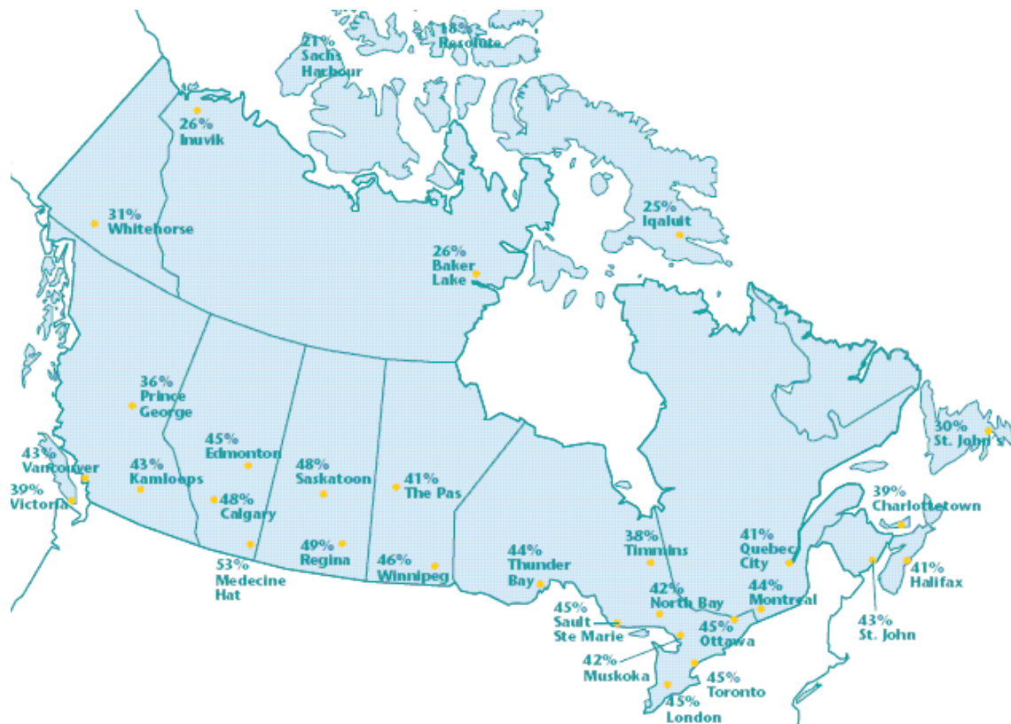
Figure 3.1 Potential Contributions of Solar Water Heaters to Energy for Water Heating in Selected Canadian Cities
